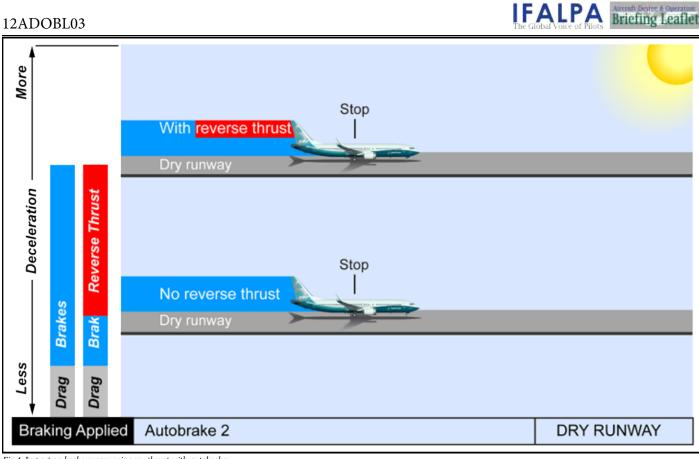
Fig 4: Impact on brake engery using rev thrust with autobrakes Data source The Boeing Company
